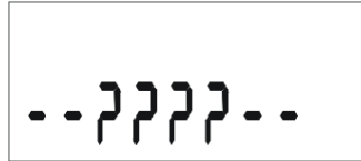
Customer interface unit in decommissioned mode
